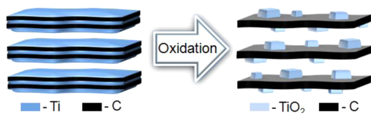
Figure 5. (a) Schematic for the oxidation of \text{Ti}_3\text{C}_2 forming nanotitania on thin sheets of carbon. Reproduced with permission from ref 88. Copyright 2014 Royal Society of Chemistry.
